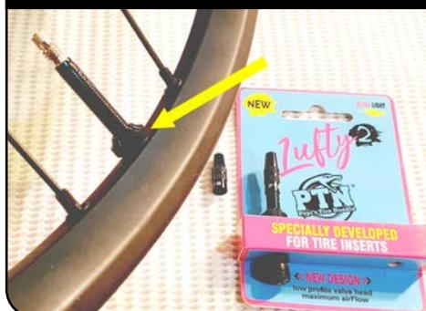
The fastening nut is tightened by hand until the valve stem is firmly anchored in the rim hole.
