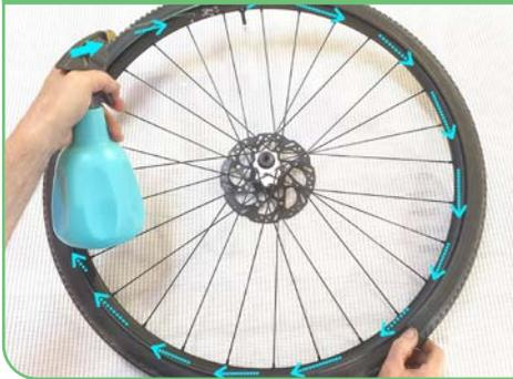
Now spray the tire side and rim wall with soapy water. This trick makes it easier for the tire to slide onto the rim.
