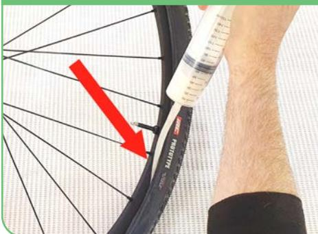
This method of filling in the sealant milk is highly recommended if the sealant milk is filled with dense granules, as it is not liquid enough to easily pass through the thin air valve shaft hole.
