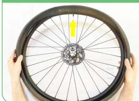
Turn the wheel so that the air valve is at the 12 o'clock position.
