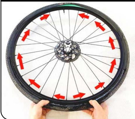
Start with hands at the 6'o clock position and push the tire into the rim, section by section. Do this with one hand on either side and push in the direction of the air valve (at the 12 o'clock position).
