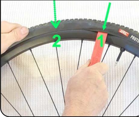
Place the tire lever next to the air valve and slide it between the tire and the rim. It's important to also press the tire with your hand to release it from the rim flank. This makes it easier to lift the tire out of the rim with the lever.
