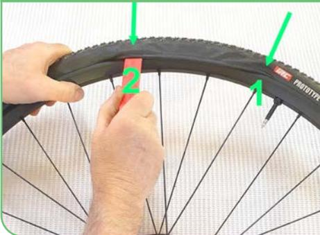
Use a second lever to lift another piece of the tire out of the rim.
