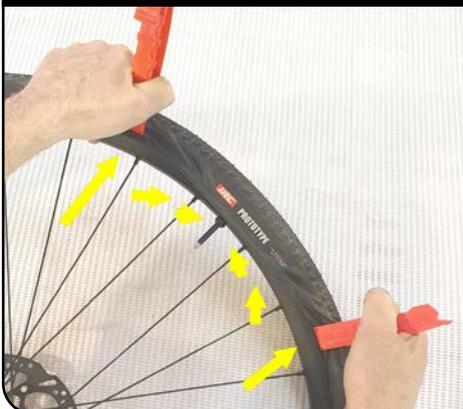
After the sealing milk is filled in, the rest of the tire can easily be pushed into the rim with the help of two tire levers.
