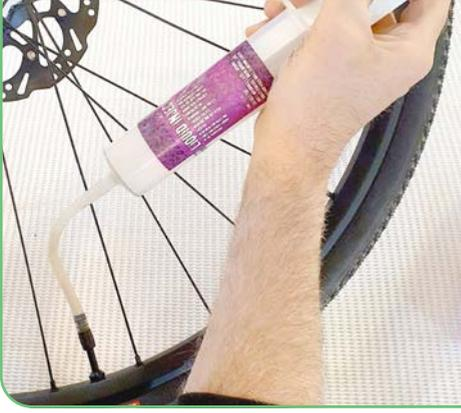
Filling the tire with a specific syringe is only recommended if the milk is very liquid, so blockages can be avoided.
