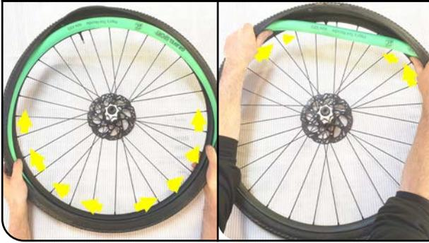
Put the PTN into the tire and slide it onto the rim bed.
